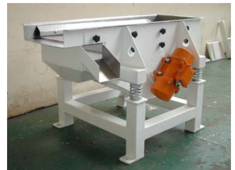
➤ This twin motor low frequency screen has two removable mesh screens fixed by "hook strip connectors". The machine separates product into 3 fractions, good product, over-size and under-size.
